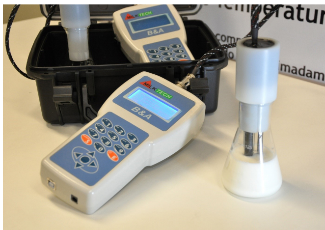
Figure 1. Milktech apparatus. It contains an electrode and a temperature sensor, so measurements are temperature compensated. The display shows the following information: Added water in % (if any) and cryoscopy. When some reconstituting is detected, the display exhibits the message: “SUSPECT”, milk added with reconstituting or high acidity.
