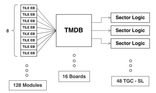
Figure 16: TileMuon System basic architecture.
