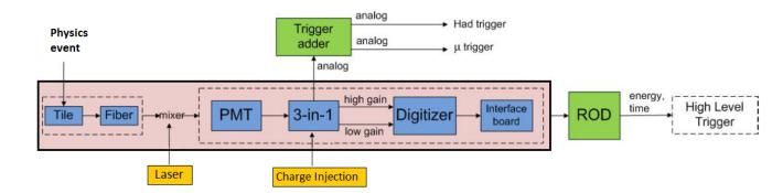
Figure 10: TileCal Readout Signal Chain (Extracted from [22]).
