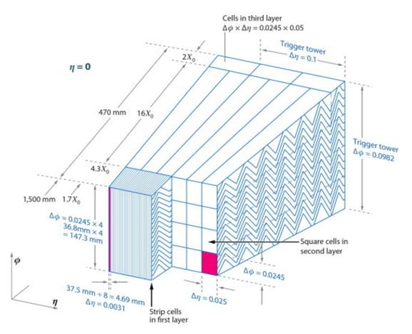
Figure 7: Segmentation of the EM calorimeter of ATLAS.((Extracted from [19])
