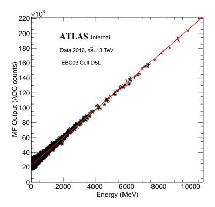
Figure 31: The TMDB calibration output estimated by Matched Filter (arbitrary units) for TileCal module EBC03 channel D5L to convert the value to MeV.
