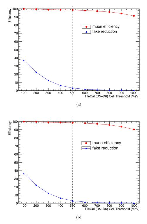
Figure 36: Muon detection efficiency and fake reduction of the Level-1 Tile-Muon Trigger as a function of TileCal cell energy sum threshold (a) A side (b) C side.
