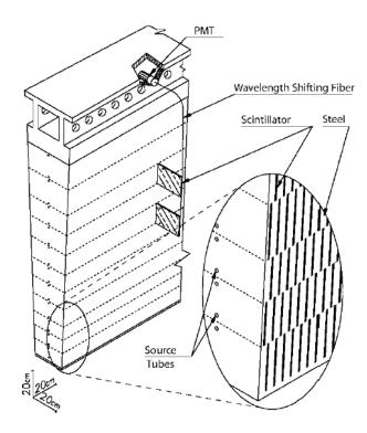
Figure 8: The Tile calorimeter design principle (Extracted from [14]).
