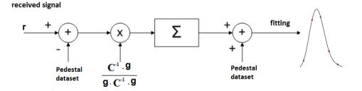
Figure 21: Signal reconstruction procedure using the Matched Filter(Extracted from [46]).
