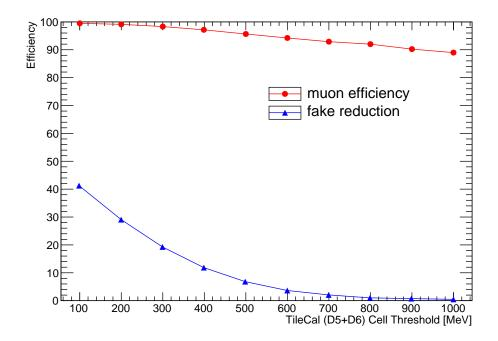
Figure 38: Muon detection efficiency and fake reduction of the Level-1 Tile-Muon Trigger as a function of TileCal cell energy sum threshold for module EBA43.
