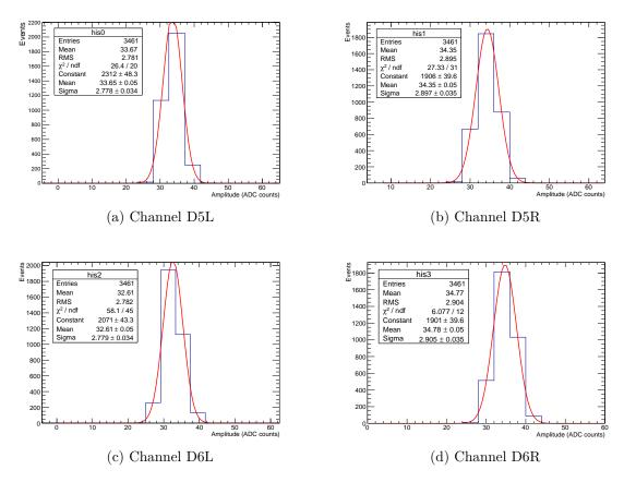
Figure 24: The noise distribution of channels from TileCal module EBA02.
