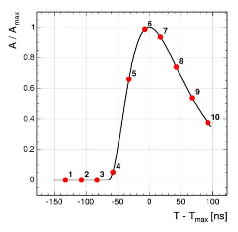
Figure 20: Typical pulse shape measured in CMS (Extracted from [45]).
