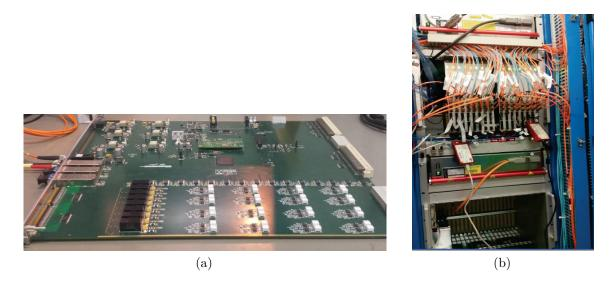
Figure 23: The TMDB hardware system: (a) the TileMuon digitalizer board. (b) the TMDB crate.
