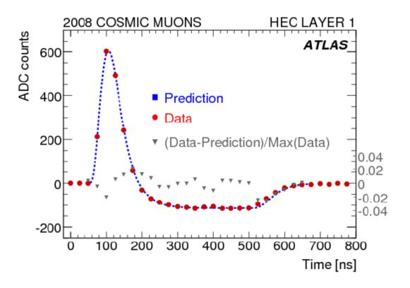
Figure 19: The LAr ionization Pulse Shape (Extracted from [44]).
