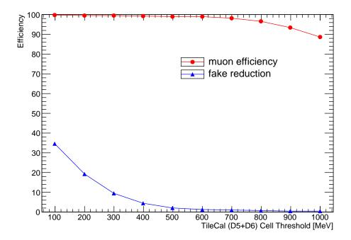
Figure 37: Muon detection efficiency and fake reduction of the Level-1 Tile-Muon Trigger as a function of TileCal cell energy sum threshold for module EBC25.
