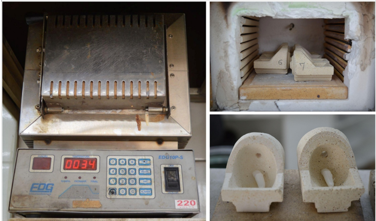
Figure 2: Demonstration of the incineration process. The image on the left shows the muffle oven at an initial temperature of 34 °C. On the right, you can see ceramic crucibles organized inside the oven. The lower right shows two samples after incineration resting at room temperature.
