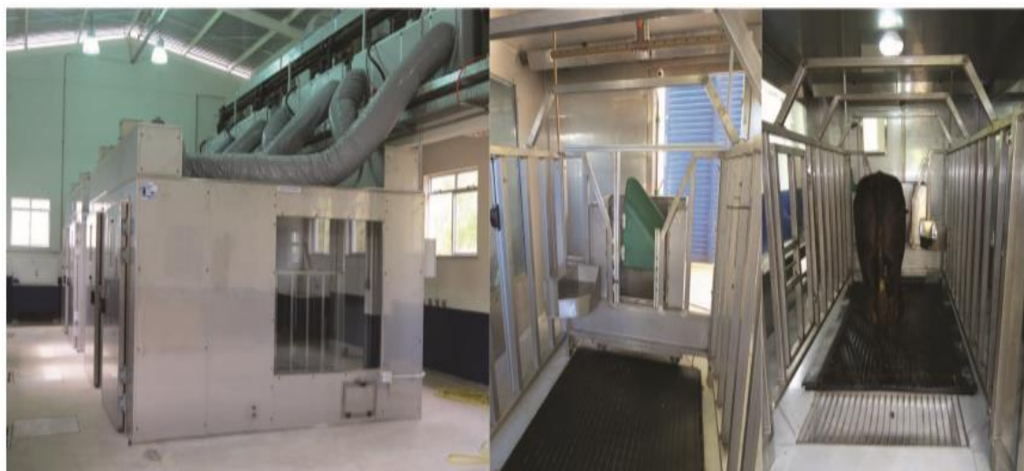
Figure 1: (A) Overview of the respiration chambers; (B) view from inside the chamber with the food and water boxes; (C) animal inside the respiration chamber (Machado et al., 2016)
