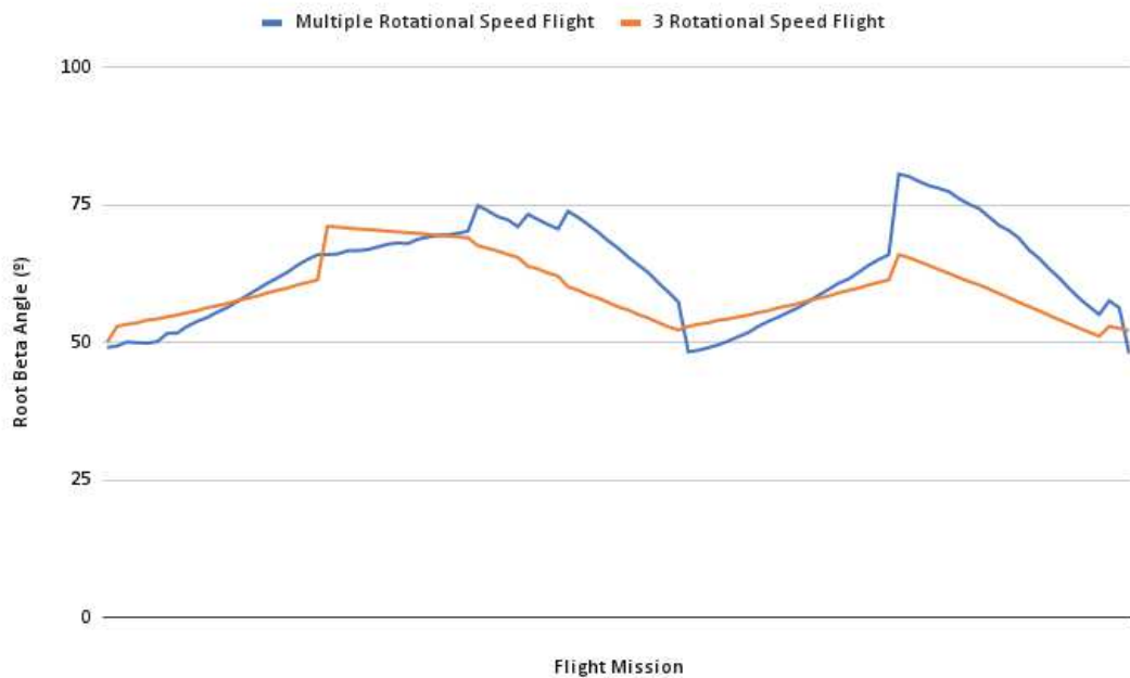
Figure 122 – Pitch Angle variation for Multi Rotational Speed Flight and 3 Rotational Speed Flight
