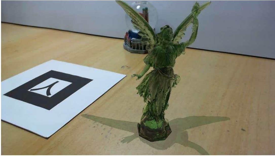
Figure 20 – Lucy model rendered with a glass material. It is possible to perceive the refraction of the snow globe through the colors in Lucy’s left wing. The texture position in skybox matches the real snow globe position.
