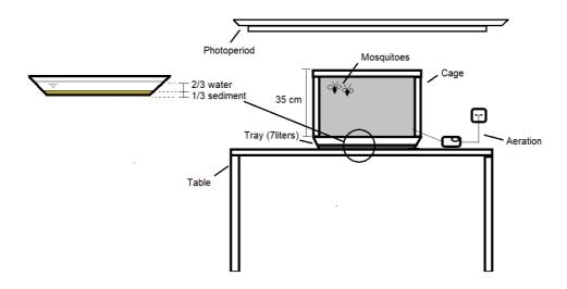
**Figure 3.4.** Schematics showing the necessary structure for *C. xanthus* establishment in laboratory cultures.
