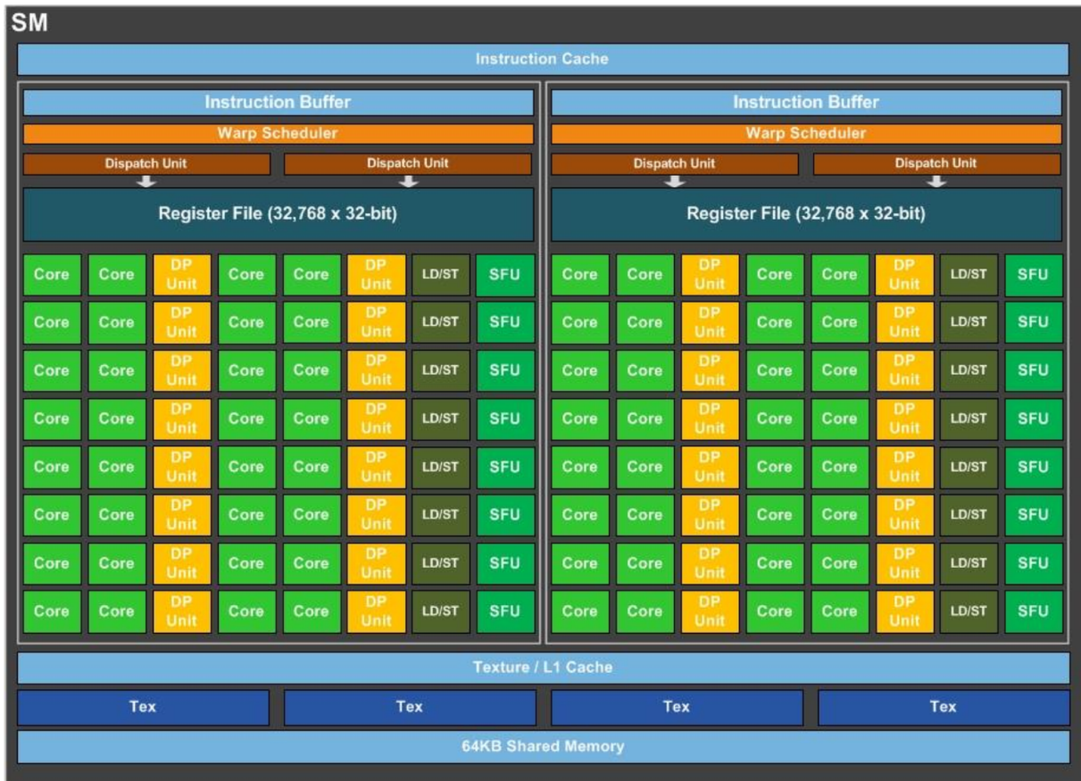
Figure 3.5: Microarchitecture of the NVIDIA Pascal (NVIDIA, 2016) streaming multiprocessor, including 64 single-precision units (cores), 16 special function units (SFUs), and 32 double-precision units (adapted from NVIDIA (2016)).
