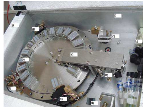
Fig. 3 Photograph of the interior of the MAI taken just before closing the apparatus. a Michelson interferometer, b sample holders on rotating disc, c light input mirror, d image exit mirror, e precision positioning system with stop and bolt, f relative position sensor that triggers the positioning bolt, g absolute position sensor that detects sample number 1, h thermometer, i isothermal box, j thermal insulation, k stock of bacteria for future experiments
