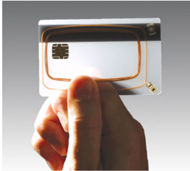
Figure 5.1: Inside an RFID card - Antenna, rfid chip, common magnetic stripe and common credit card chip.
