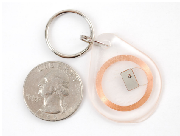
Figure 5.2: A coin size RFID keyring with antenna and micro-chip inside.
