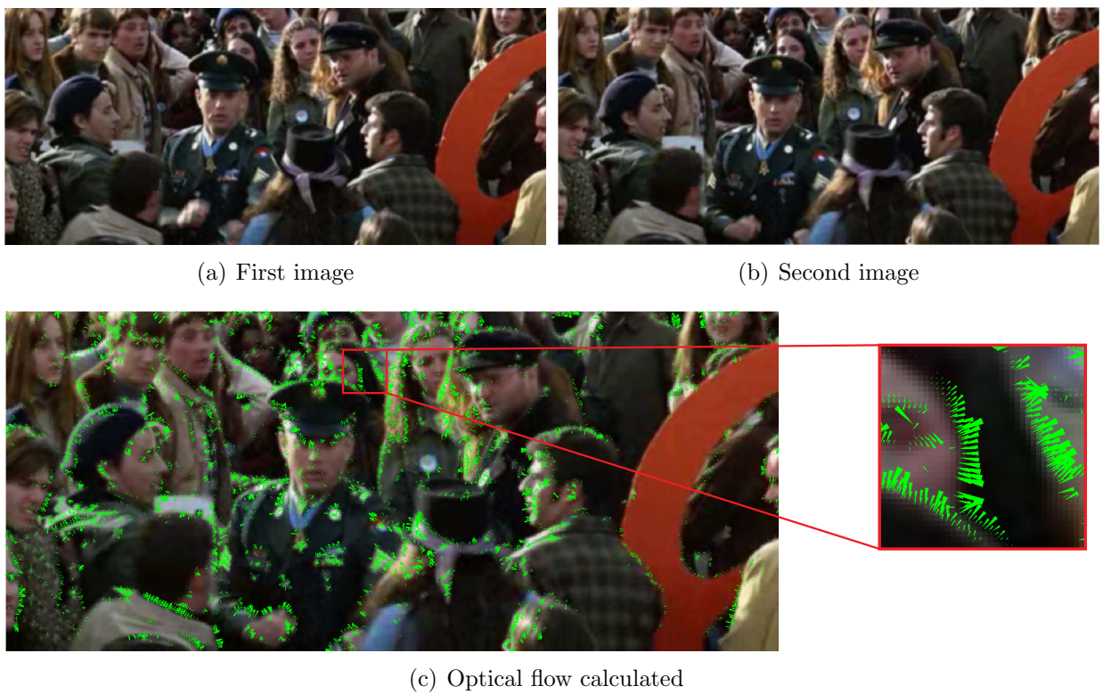
Figure 4.1: Optical flow detected by our method.
