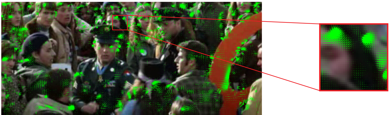
Figure 4.2: Optical flow detected using Horn and Schunck method (HORN; SCHUNCK, 1981).
