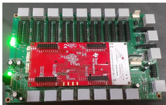
(c) Placa de controle Motherboard DSPMB_Launchxl_F28379D_V1 com kit LAUNCHXL-F28379D, baseada no DSP TMS320F28379D.
