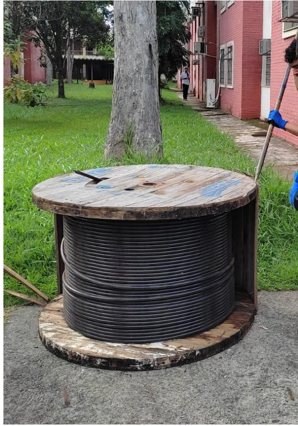
Figura 11 – The multiconductor spool with 1000 m used in the laboratory measurement campaign.
