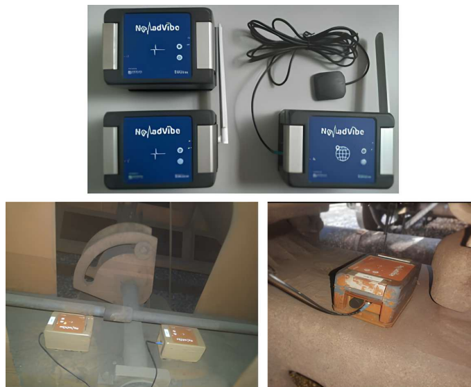
Figure 26 – Inertial sensor modules installed on the railway vehicle, including placements on the carbody, leading bogie, and trailing bogie.
