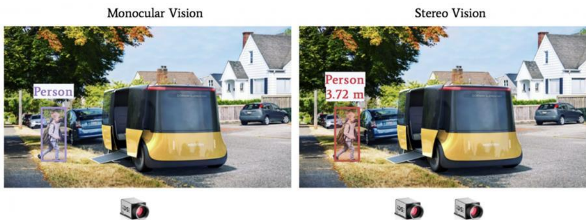
Figure 3 - Difference from monocular to stereo vision
