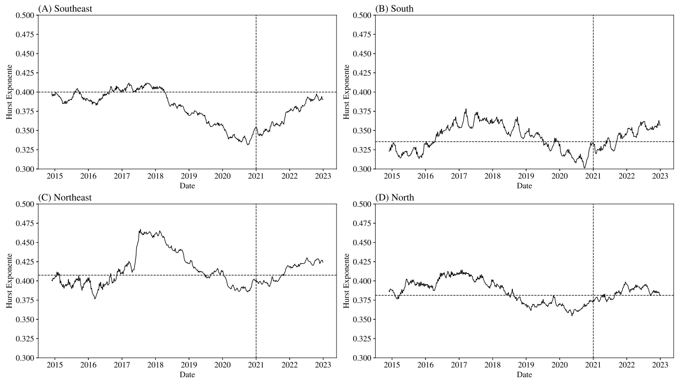
FIGURE 7. The graphs present the dynamic behavior of the Hurst coefficient ( H_2 ) for the four submarkets using a window of 702 weeks and a unit step. The dashed vertical line indicates when there was a transition in how the price was calculated, with the introduction of the hourly hydrothermal dispatch model on January 1, 2021. Before this date, the price was calculated weekly through a weekly hydrothermal dispatch model. From this landmark, the weekly price started to be obtained by the arithmetic average of the hourly prices throughout the week. The dashed horizontal line represents the value of H_2 calculated for the complete series, as presented in Table 3.
