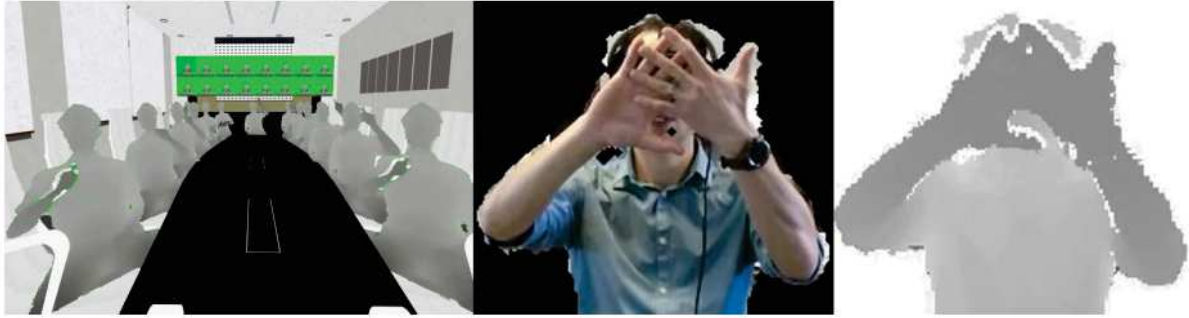
Figure 11 - 16 user streams in a VRComm Virtual Experience (left) and RGBD user transmission of RGB-part (middle) and depth-part (right) (10)
