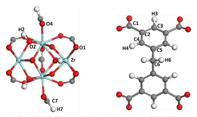
Figure S8. Labels of the atoms for the inorganic and organic parts of MIP-200(Zr).
