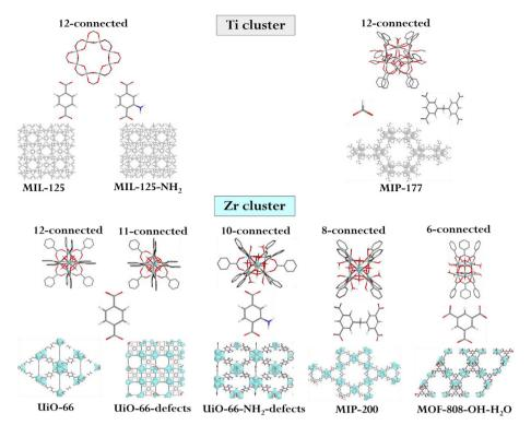
Fig. 1. Illustrations of the inorganic Zr and Ti building blocks present in a few representative 3D-MOFs considered in this work.
