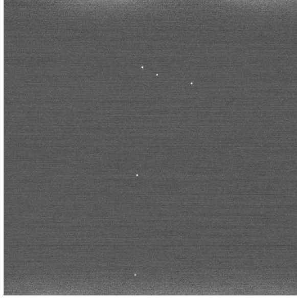
Figure 26 – Example of an image acquired during a ^{55}\text{Fe} Daily Calibration run.
