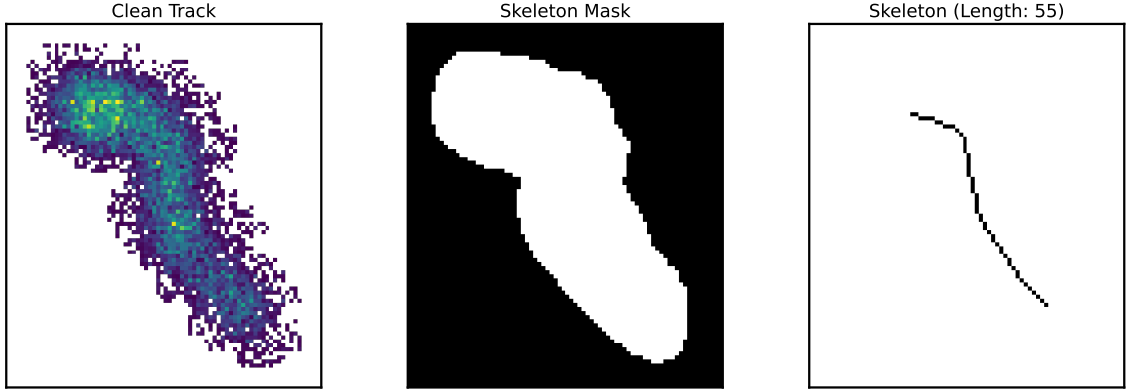
Figure 19 – Skeletonization process: from the processed track mask to the one-pixel-wide backbone.
