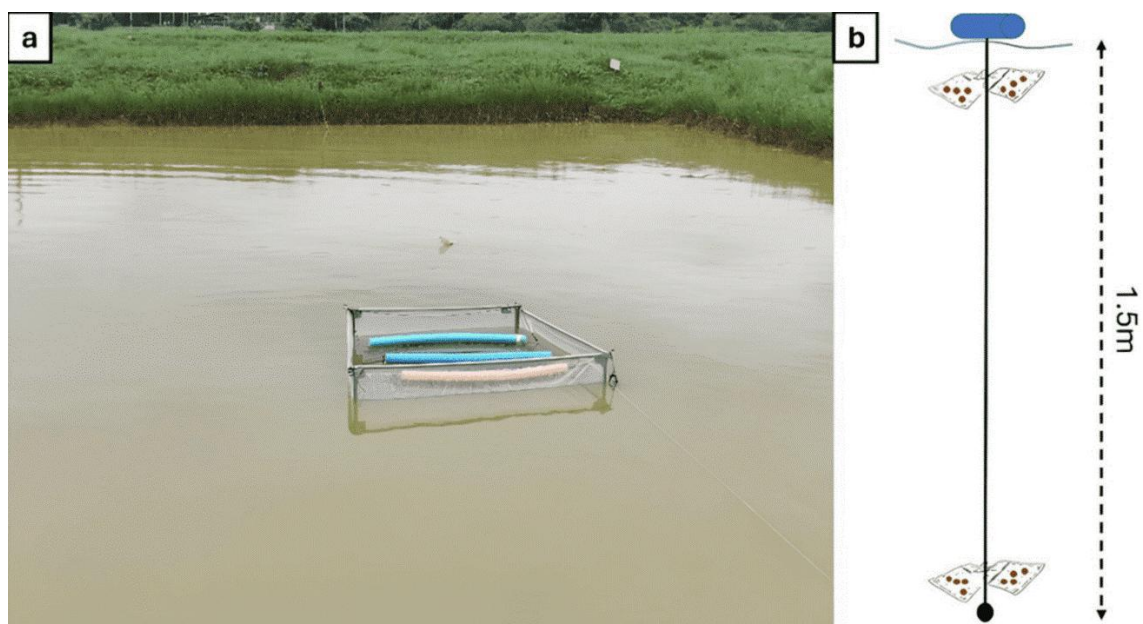
Fig. S1: Feed degradation experiment. (a) Surface view of the in-situ experiment; (b) schematic representation of a single replicate, illustrating the spatial organization of components, including feed placement, used to monitor breakdown.
