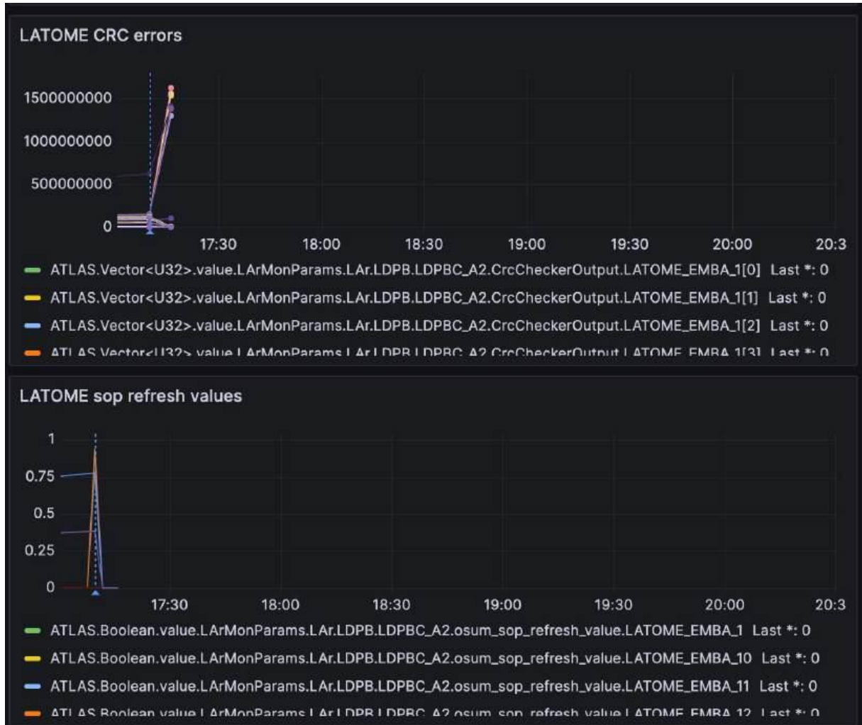
Figure 53 – Evolution of CRC errors and sop_refresh values over time. The drop in errors aligns with the moment the sop_refresh signal is set to zero.
