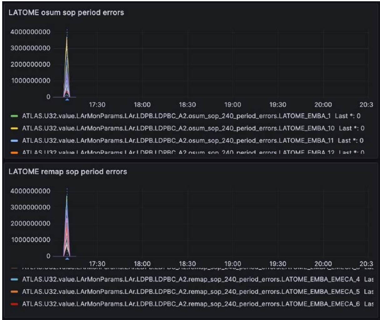
Figure 52 – SOP period error counters for the REMAP and OSUM blocks during ATLAS online testing. Errors are observed at startup but converge to zero after sop_refresh is disabled.
